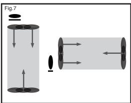
The most commonly used technique for painting a large surface is the 'crisscross' technique, i.e. you apply the product in a horizontal strips and then cross over these strips by applying the product in a vertical strips (Fig.7).
